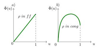
Fig. 7. FD as a function of u: a) monotonic dependence for a fixed  $\rho$  in free-flow; b) concave dependence for a fixed  $\rho$  in congested regime.
