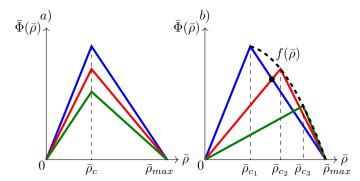
Fig. 6. Fundamental diagrams and their dependence on speed limits: a) monotonic dependence  $\partial \bar{\Phi}(\xi, \eta, \bar{\rho}, u)/\partial u > 0$  used in [38]; b) dependence we assume here, i.e., possible increase of  $\rho_c$  for larger speed limits (from real data, see [28]). Blue line: u = 1. Red line: u = 0.7. Green line: u = 0.5. Bold dashed line: maximal flow function defined in (39).
