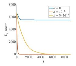
Fig. 5. L<sub>1</sub> error as a function of time for different control gains.
