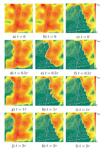
Fig. 4. Traffic control in Grenoble downtown. Right column: desired density  $\rho_d(x, y, t)$ ; middle column: evolution of  $\rho(x, y, t)$  with  $k = 5 \cdot 10^{-5}$ ; left column: evolution of  $\rho(x, y, t)$  with k = 0. All the plots represent snapshots made at: a), b) c) t = 0; d), e), f)  $t = 0.5\tau$ ; g), h), i)  $t = 1\tau$ ; j), k), l)  $t = 2\tau$ . The color bar denotes the ratio of the current density to the the maximal density all over the network.
