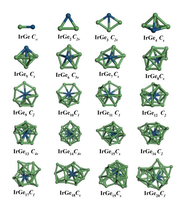
Figure 1. Most stable structures for  $IrGe_n$  clusters (n=1-20) together with their spatial symmetry group.
