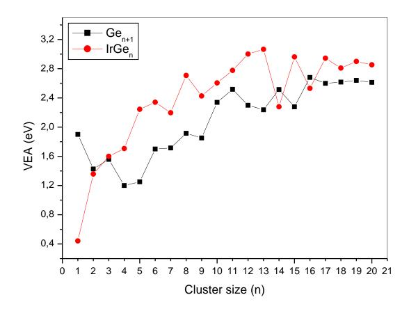
**Figure 6.** Vertical electron affinity VEA (eV) of the lowest-energy structures of  $Ge_{n+1}$  [30] and IrGe<sub>n</sub> (n=1-20) clusters.
