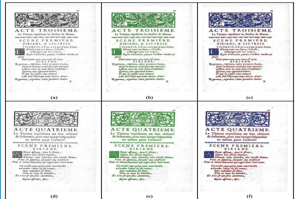
Example of document segmentation. {(a), (d)} are the original images of the same book, {(b), (e)} are the results of the foreground pixel extraction using an adapted Hierarchical Ascendant Classification and {(c), (f)} are the final results of clustering steps.
