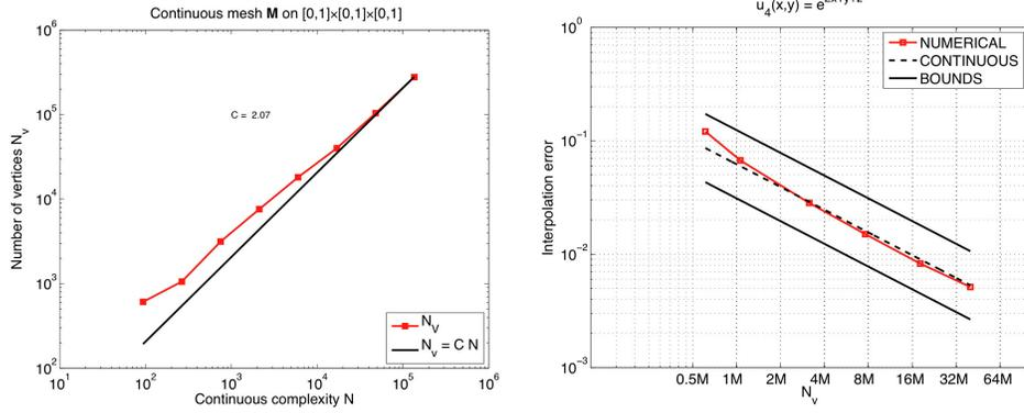
FIG. 1.6. *Left, comparison between the continuous mesh complexity and the number of vertices for a sequence of unit meshes  $\{\mathcal{H}_{3,\alpha}\}_\alpha$  with respect to  $\{\mathbf{M}_3(\alpha)\}_\alpha$  on  $\Omega_3$ . Right, comparison between the continuous interpolation error  $\|u_4 - \pi_{\mathcal{M}_{3,\alpha}} u_4\|_{\mathbf{L}^1(\Omega_3)}$  and the discrete interpolation error  $\|u_4 - \Pi_h u_4\|_{\mathbf{L}^1(\Omega_{3,h})}$ .*
