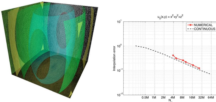
FIG. 1.7. Left, iso-surfaces of function  $q$ . Right, comparison between the continuous interpolation error  $\|u_5 - \pi_{\mathcal{M}_{4,\alpha}} u_5\|_{\mathbf{L}^1(\Omega_4)}$  and the discrete interpolation error  $\|u_5 - \Pi_h u_5\|_{\mathbf{L}^1(\Omega_{4,h})}$ . In this case, the continuous interpolation error is computed numerically by means of the linear approximation of the continuous mesh on a fine uniform discrete mesh.
