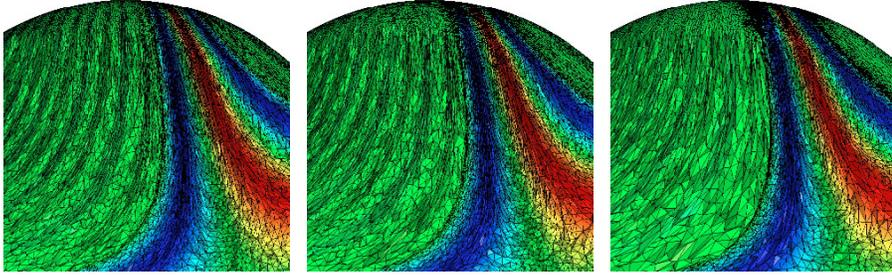
FIG. 3.4. Optimal anisotropic adapted meshes for the  $\mathbf{L}^1$  (left),  $\mathbf{L}^2$  (middle) and  $\mathbf{L}^\infty$  (right) norms for a complexity equal to 275 000. Views of the volume mesh in a cut plane.
