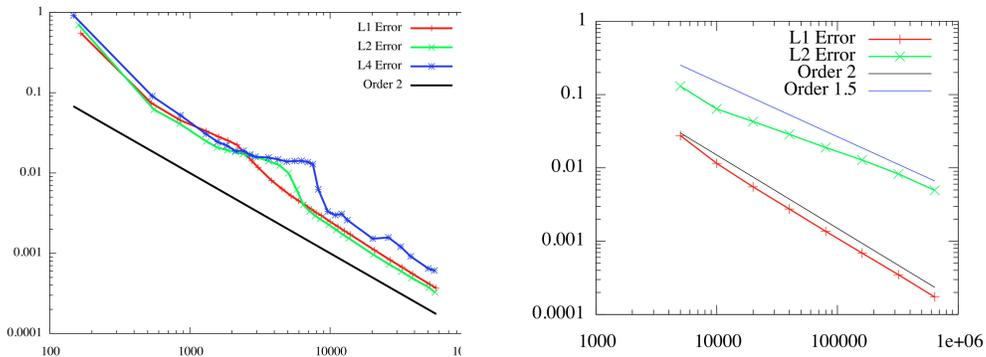
FIG. 3.2. Plot of the linear interpolation error (ordinate) with respect to the number of vertices (abscissa) for functions  $f_1$  (left) and  $f_2$  (right). The order of convergence is also represented.
