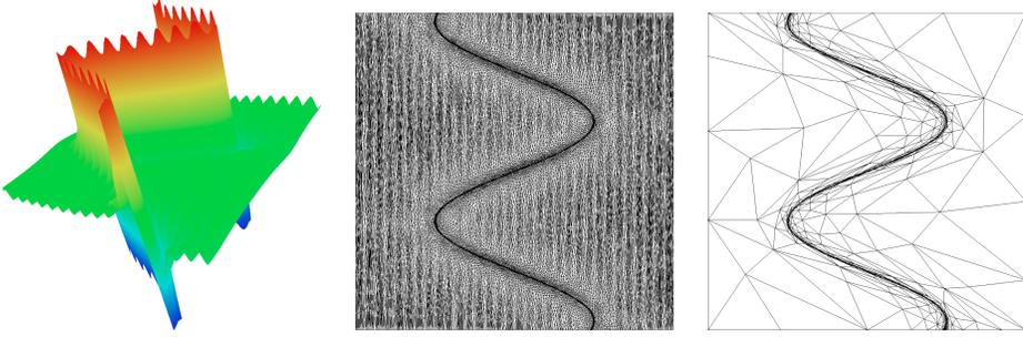
FIG. 3.3. Left, representation of function  $f_2$ . Optimal adapted meshes, composed of almost 100 000 vertices, controlling the interpolation error in  $\mathbf{L}^1$  norm (middle) and in  $\mathbf{L}^\infty$  norm (right).
