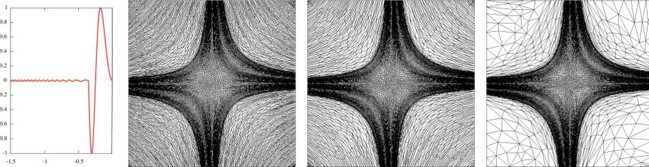
FIG. 3.1. From left to right, representation of function  $f_1$  along the cut line  $y = 0$ , optimal adapted meshes for norms  $\mathbf{L}^1$ ,  $\mathbf{L}^2$  and  $\mathbf{L}^4$ . Each mesh is composed of about 7 000 vertices.
