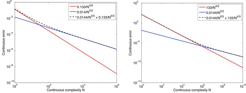
FIG. 1.1. *Left, convergence history obtained for the function  $u_3$  on the set of inhomogeneous continuous meshes spans by  $\mathbf{M}_2(\alpha)$  defined on  $\Omega_2$ . Right, convergence history for the error function of Remark 1. In that specific case, the coefficients involved in the error expression lead to observe  $O(N^{-\frac{4}{3}})$  as predominant term in the reachable range of complexity  $[1, 10^6]$  whereas the asymptotic convergence order is  $O(N^{-\frac{2}{3}})$ .*
