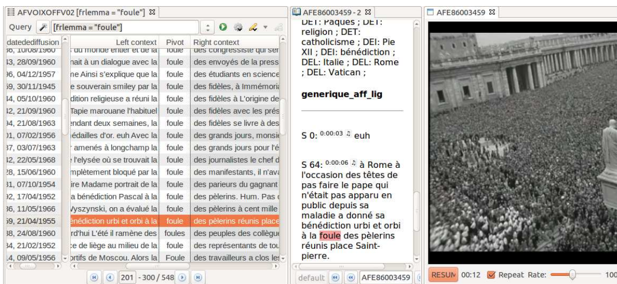
Figure 7. Hyperlinked windows managing results associated with the word “foule” (crowd): CONCORDANCE (left window), transcript EDITION (middle window) and synchronized video playback (right window)
