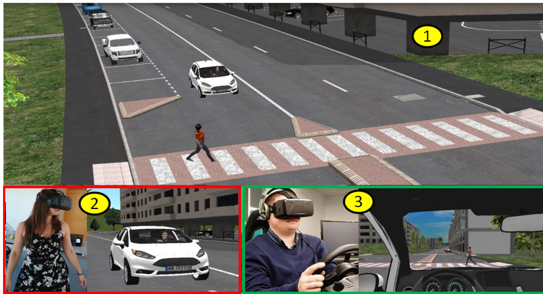
Figure 3: Illustration of an example of scenario implemented on the V-HCD platform to study the interactions between a pedestrian and an AV with a more or less attentive driver.
