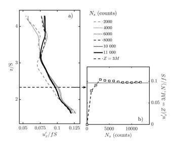
Fig. 6: Statistical convergence of  $u'_x$  profiles for the example of the XG10 case. a) Profiles of  $u'_x/fS$  versus z/S for various  $N_s$ . b) Values of  $u'_x$  extracted at  $z=3M \simeq 2.3S$  from these profiles and additional ones at other  $N_s$  values (not shown in a)), as a function of  $N_S$ .
