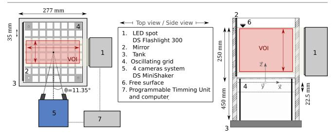
Fig. 1: Sketch of the experimental setup
