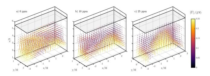
Fig. 8: Mean flow 3D Eulerian velocity fields  $\overline{U}$  coloured by the velocity magnitude  $\left|\overline{U}\right| = \sqrt{\overline{U}_x^2 + \overline{U}_y^2 + \overline{U}_z^2}$  for water (a),  $C_{XG} = 10$  ppm (b) and  $C_{XG} = 25$  ppm (c).
