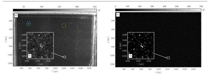
Fig. 3: Example of particle image from camera 1, water run, before (a,b) and after pre-treatment (c,d). b) and d) are zooms of respectively a) and c) on the same group of particles. Dashed circles stress the location of a dust particle crossing the VOI (blue, mixed) and of a shaded spot on the camera sensor (orange, dashed) efficiently removed by the pre-treatment.
