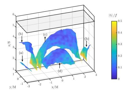
Fig. 10: Isosurface of vertical mean velocity  $\overline{U}_z$  scaled by fS at values -0.25 (a), -0.075 (b), 0.075 (c) and 0.25 (d) (XG25 case). Black arrows point the corresponding surface and indicate the vertical velocity direction (up for  $\overline{U}_z > 0$ , down otherwise). The gray rectangle denotes the location of the free surface. Surface are colored by the local shear rate magnitude  $|\dot{\gamma}|$  made non dimensional dividing by f.
