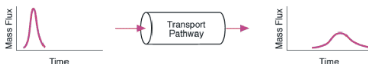
Figure 7: Scheme of a compartment capturing a solute transport process in the lumped-parameter model sense (Golder Associates, 2014).
