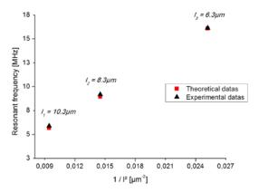
Figure 2: Plot of the fundamental mode resonant frequencies of  $2.4\mu m$  wide cantilevers with three different lengths l showing the linear dependence on  $1/l^2$ . Theoretical datas (red) are obtained from finite element modeling. Experimental datas are obtained under external actuation and sensing configuration at
