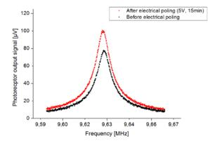
Figure 3: Fundamental mode resonant frequency of a 2µm wide and 10.2µm long cantilever before (black curve) and after (red curve) poling of the PZT thin film. Measurements are achieved according to the integrated actuation (12.6mV AC voltage is applied) and external sensing configuration, at room temperature and under secondary vacuum (9.8.10<sup>-7</sup> mbars). Each datas curve has been averaged 10 times. The structure exhibits a quality factor of 1150 at 9.63MHz.
