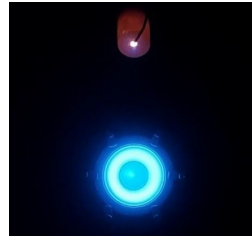
Figure 2. Front view of the ISCT200 firing with xenon. The 5-A cathode is located above the thruster body.
