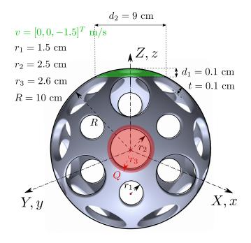
Figure 23: Spherical ball: problem setup
