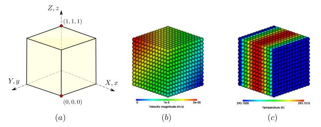
Figure 2: Linear thermo-elasticity: (a) geometry and the initial conditions for (b) velocity and (c) temperature.
