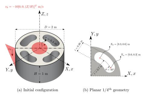
Figure 15: Punch test: problem setup
