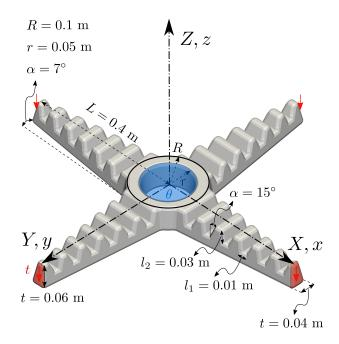
Figure 20: Gripper: problem setup
