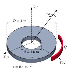
Figure 10: Rotating disk configuration
