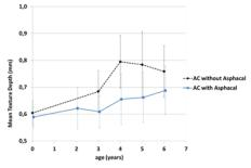
**Fig. 1.** Mean Texture Depth as a function of pavement age for the 20 sections built in 2011-13 based on BBSG with or without Asphacal<sup>®</sup> hydrated lime in the Vosges Département.
