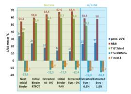
**Fig. 2.** Rheological properties for the neat initial bitumen, the same binder after laboratory aging (RTFOT and RTFOT+PAV) and the binder extracted from A84 sections after 5 yrs.
