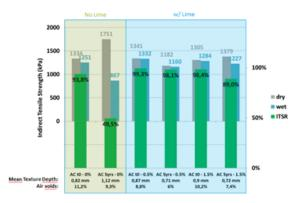
**Fig. 3.** Indirect Tensile Strength (ITS) for the initial mixtures and after 5 yrs. The ratio (ITSR) between dry and wet ITS is also given. Void content and Mean Texture Depth are also given.
