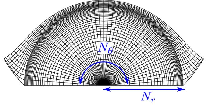
Fig. 2. Radial and angular parameters of mesh refinement.
