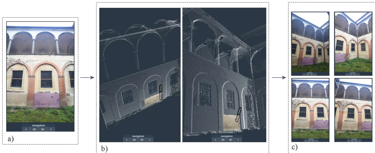
Figure 4. Processing steps via Aioli: (a) selection of the annotation on the first image, (b) detection of 3D points corresponding to the selection and (c) propagation of the annotation on the other images of the set
