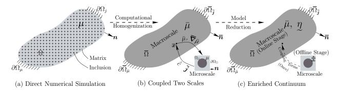
Figure 2: Schematic representation of the development of the enriched continuum formulation: by performing computational homogenization: the DNS problem (a) is replaced by the coupled two-scale problem (b), followed by a model reduction on the micro-scale to obtain an enriched continuum formulation (c).
