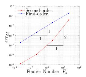
Figure 6: Error analysis for the local time integration schemes, to be used with the internalvariable method. The one step second-order accurate time integrator, equation (18) reveals a higher accuracy than the first-order backward-Euler time integrator, (19). The expression for  $err_{\Delta t}$  is given in equation (36).
