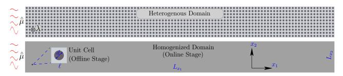
Figure 3: Problem settings: Top: a heterogeneous domain with 1000 unit-cells. 100 in  $x_1$ direction and 10 in  $x_2$ -direction. Bottom: corresponding homogenized domain for the solution of the enriched continuum formulation. The unit-cell shown inside is used to obtain the coupling terms in equations (11) and (12) in the off-line stage. The material properties and geometrical parameters are provided in Table 1.
