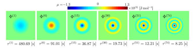
Figure 4: The selected enrichment-functions  $\Phi^{(k)}$  obtained by solving the generalized eigenvalue problem (44). An associated decay/rise time  $\tau^{(k)} = 1/\alpha^{(k)}$ , with  $\alpha^{(k)}$  the k-th eigenvalue, is also given for each enrichment function  $\Phi^{(k)}$ .
