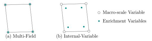
Figure 1: Spatial discretizations schemes for the enriched-continuum. (a) Multi-field: both the macro-scale and enrichment-variables are interpolated using bi-linear quadrilateral finite elements. (b) Internal-variable: the macro-scale variable is interpolated by bi-linear quadrilateral finite elements while the enrichment-variables are computed at the Gauss quadrature points.
