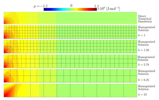
Figure 8: The chemical potential field  $\mu$  in the heterogeneous domain (top plot) obtained by the direct numerical simulation (DNS). The homogenized chemical potential field  $\bar{\mu}$  obtained by enriched continuum formulation solved using multi-field method with increasing homogenization levels h (from the second plot to the bottom).
