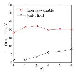
Figure 10: Computational time for the internal-variable and multi-field method for increasing number of enrichment-variables  $\eta^{(q)}$ .
