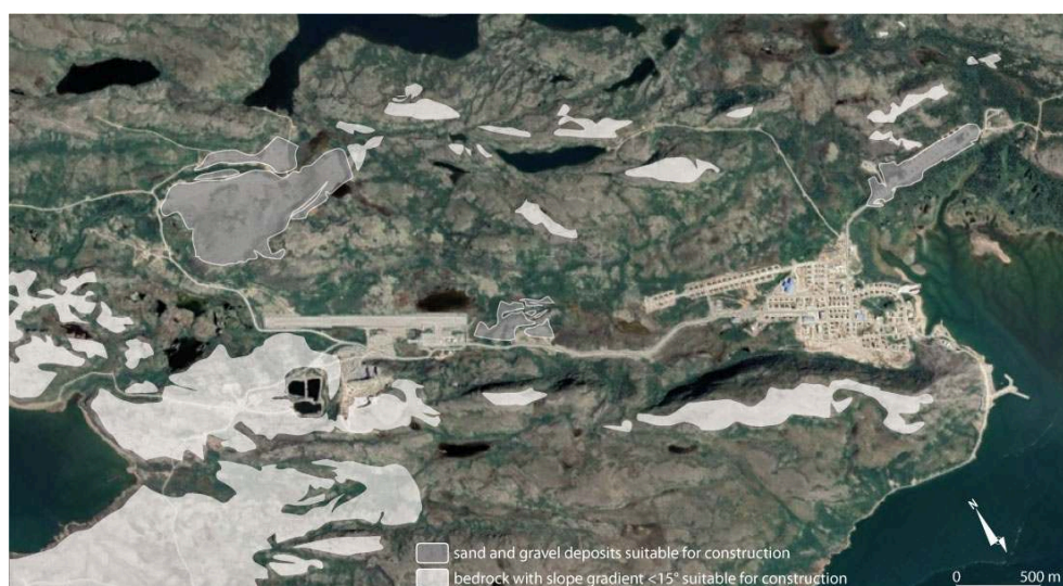
Figure 8 – Location of the suitable construction areas on surfaces where permafrost thawing and active layer fluctuations have little effect on the stability of the surface, away from active slope processes areas (modified from Aubé-Michaud et al., 2017).
