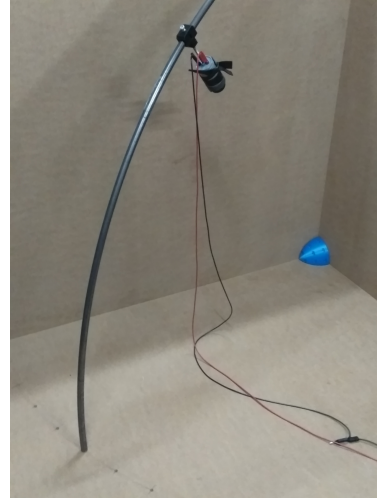
Figure 5: Experimental layout: The SFMA is placed at the corner of 3 wooden panels mounted in a anechoic room. A loudspeaker can move on a eighth of a 1 m radius spherical surface, centered on the corner.
