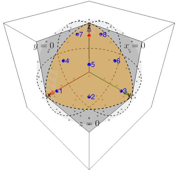
**Figure 1:** One eighth of a spherical Gauss-Legendre mesh for  $L = 5$ . The full sphere mesh is shown as the union of gray, blue and red nodes; the eighth of spherical mesh as the union of blue and red node. The mesh used for the SFMA prototype is shown in blue. The eighth of spherical fraction is shown in orange and the rigid bounding planes  $x = 0$ ,  $y = 0$  and  $z = 0$  are shown in gray.
