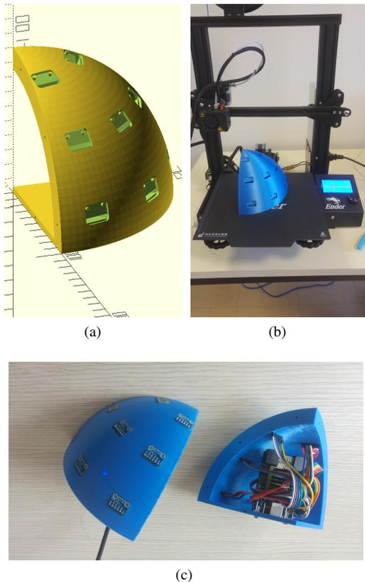
**Figure 4:** One eighth of a sphere SFMA design and building. (a) Spherical shell design on OpensCAD software. (b) The spherical shell built using a FDM 3D printer. (c) The SFMA prototype with MEMS microphones and USB streamer embedded.
