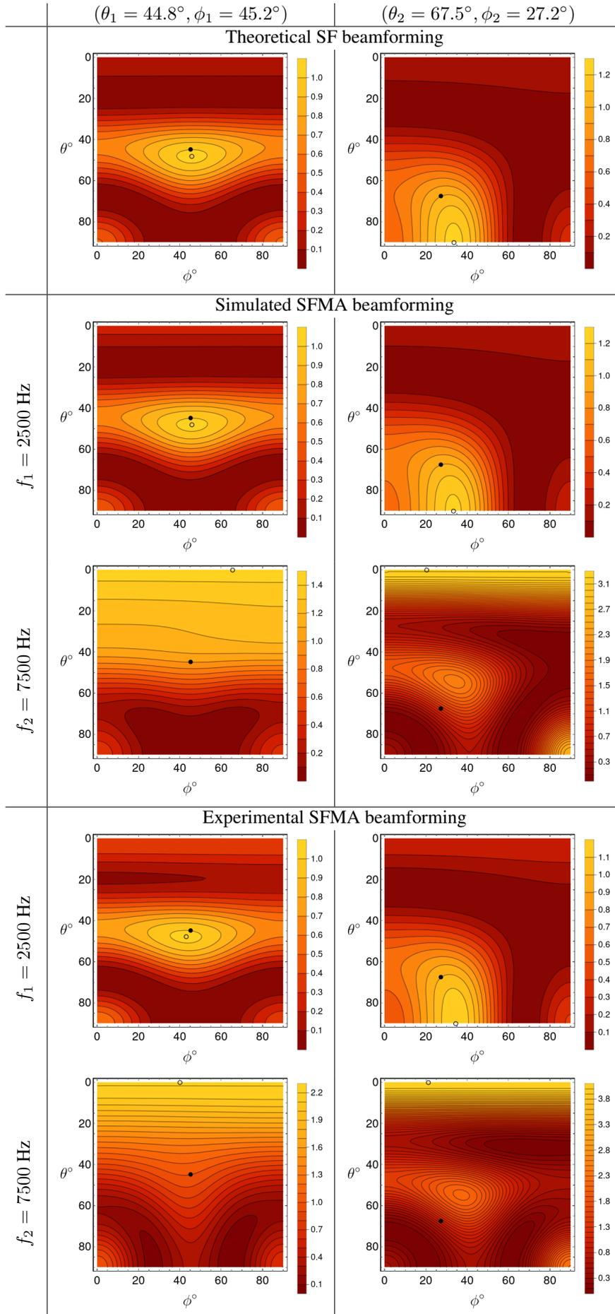
**Figure 6:** Beamforming results for two source source DOA  $(\theta_1 = 44.8^\circ, \phi_1 = 45.2^\circ)$  and  $(\theta_2 = 67.5^\circ, \phi_2 = 27.2^\circ)$  and the frequencies  $f_1 = 2500$  Hz and  $f_2 = 7500$  Hz. The normalized squared beamformer output  $|y(\theta, \phi)|^2/|y(\theta_{1,2}, \phi_{1,2})|^2$  is plotted for all possible steering directions  $(\theta, \varphi) \in (0^\circ, 90^\circ) \times (0^\circ, 90^\circ)$ .
