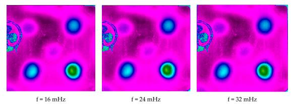
**Figure 18.** Amplitude images of the calculated harmonic response (at f = 16m Hz, f = 24 mHz and f = 32 mHz).
