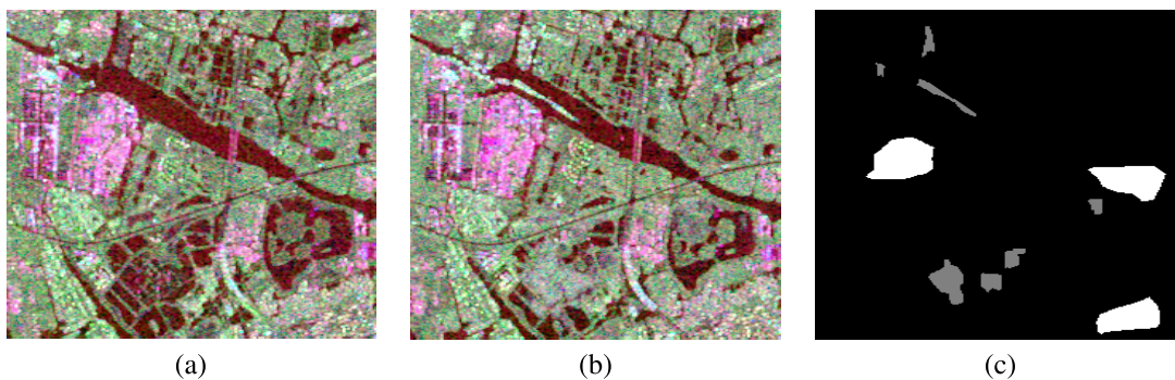
Fig. 5. Pauli RGB ( R = HH + VV , G = HV , and B = HH - VV ) of quadpol RADARSAT-2 images captured over Suzhou city, East China on (a) April 9, 2009 and (b) June 15, 2010, multilooked with 24-looks. (c) Truth change map. The white means no-change, the gray means change, and the black means unlabeled pixels.
