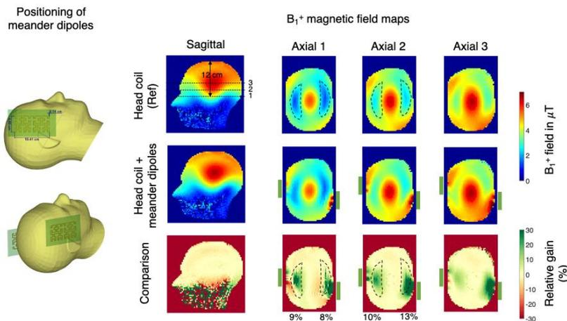
Fig. 2. Position of the meander dipoles (left) and  $B_1^+$  field distribution maps of the head coil alone (top right) and coupled with the resonant meander dipoles (middle right) in sagittal and axial orientations. The bottom right row shows the relative gain between meander dipoles and reference map.
