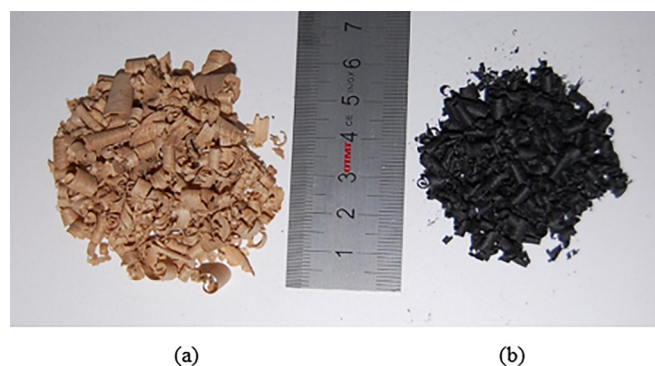
FIG. 1. Photographs of samples: (a) in the initial state, wc_{s1} , and (b) after pyrolysis at 573 K, wc_{s2} .
