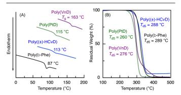
**Fig. 4.** Differential scanning calorimetry (DSC) (A) and thermogravimetric analysis (TGA) (B) curves of poly((–)-VnD) ( $M_n$  = 17000), poly(PtD) ( $M_n$  = 20000), poly((±)-HCvD) ( $M_n$  = 26500), and poly(β-Phe) ( $M_n$  = 90000).
