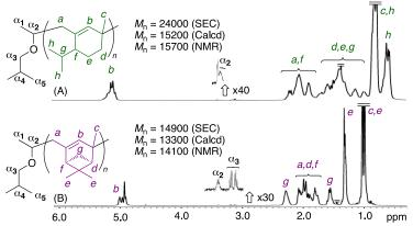
Fig. 3.  $^{1}H$  and  $^{13}C$  NMR spectra (in CDCl<sub>3</sub> at 55  $^{\circ}C$ ) of poly(PtD) and poly((-)-VnD) obtained in cationic polymerization: [M]<sub>0</sub>/[2]<sub>0</sub>/[SnCl<sub>4</sub>]<sub>0</sub>/[nBu<sub>4</sub>NCl]<sub>0</sub> = 100/1.0/5.0/4.0 mM in toluene/CH<sub>2</sub>Cl<sub>2</sub> (50/50 vol%) at -78  $^{\circ}C$ .
