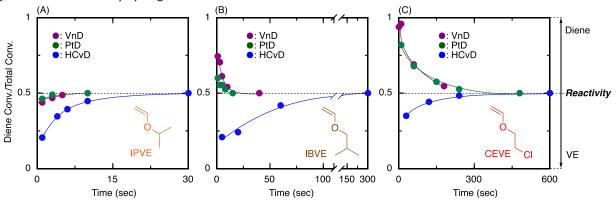
Fig. 7. Plots of diene conversion in total monomer conversion vs. time in living cationic copolymerization of *exo*-methylene conjugated dienes and vinyl ethers: [diene]<sub>0</sub>/[VE]<sub>0</sub>/[2]<sub>0</sub>/[SnCl<sub>4</sub>]<sub>0</sub>/[nBu<sub>4</sub>NCl]<sub>0</sub> = 100/100/1.0/5.0/4.0 mM in toluene/CH<sub>2</sub>Cl<sub>2</sub> (50/50 vol%) at -78 °C.
