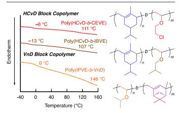
Fig. 10. DSC curves of the polymers obtained in the block copolymerization of  $(\pm)$ -HCvD or (-)-VnD with VEs.
