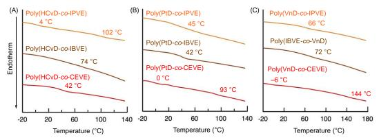
Fig. 8. DSC curves of the copolymers obtained in living cationic copolymerization of  $(\pm)$ -HCvD (A), PtD (B), or (-)-VnD (C) with various VEs.  $M_n = 36600$  (poly(HCvD-co-IPVE)), 23500 (poly(HCvD-co-IBVE)), 27600 (poly(HCvD-co-CEVE)), 31300 (poly(PtD-co-IPVE)), 26000 (poly(PtD-co-IBVE)), 24400 (poly(PtD-co-CEVE)), 19200 (poly(VnD-co-IPVE)), 17300 (poly(VnD-co-IBVE)), 17700 (poly(VnD-co-CEVE)).
