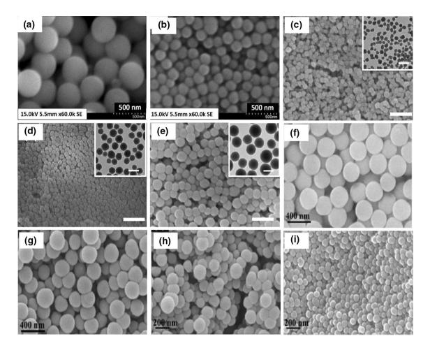
**Fig. 6** Scanning electron microscopy (SEM) of silica nanoparticles with fixed concentration of tetraethylorthosilicate (TEOS) and varied ethanol to water ratios: **a** 4:1, **b** 3:1 (Prabha et al. 2019). Fixed concentration of TEOS, ethanol and water and varied NH<sub>3</sub> concentrations: **c** 150 mM, **d** 200 mM, **e** 250 mM, reprinted with permission from Zhang et al. (2016). Fixed concentration of NH<sub>3</sub> and ethanol
