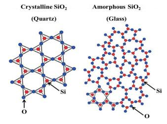
Fig. 1 Structure of crystalline and amorphous silica
