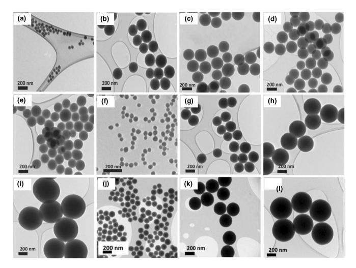
**Fig. 7** Transmission electron microscopy (TEM) of silica particles. **a–d** fixed concentration of tetraethylorthosilicate (TEOS), ammonia solution (NH<sub>4</sub>OH) and varied amounts of water. Fixed concentration of TEOS and water, and varied concentration of NH<sub>4</sub>OH **f** 0.11 M, **g** 0.28 M, **h** 0.57 M, **i** 1.13 M, **j** 0.17 M, **k** 0.40 M, **l** 0.85 M, reprinted
