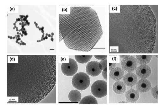
**Fig. 12** Transmission electron microscopy (TEM) of **a** mesoporous silica nanoparticle with an average diameter of 120 nm. **b** High-resolution image of a single particle, pore size 2.7 nm, reprinted with permission from Yu et al. (2011). **c** 0.1 M CTAB:45 M H<sub>2</sub>O pore size 2.9 nm. **d** 0.1 M CTAB:45 M H<sub>2</sub>O pore size 2.7 nm, reprinted with permission from Vazquez et al. (2017). **e** Gold–mesoporous silica
