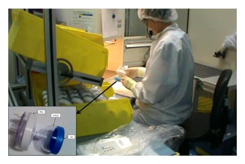
Figure 1: Workstation dedicated to filter cleaning and description of the filter.
