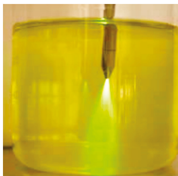
Figure 6. Tyndall effect, 10 ppm fluorescein sodium in water [4].
