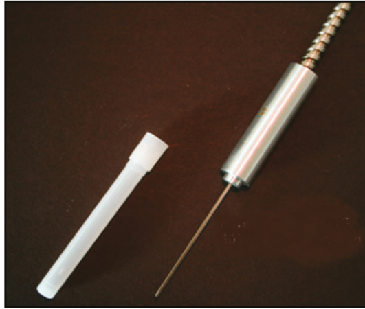
Figure 5. Cannula sterican 19G, 30° bevel [4].
