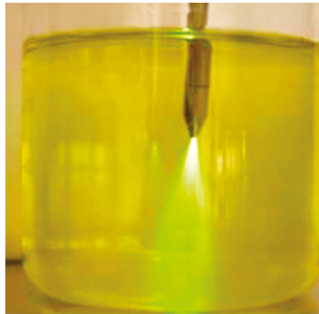
Figure 6. Tyndall effect, 10 ppm fluorescein sodium in water [4].
