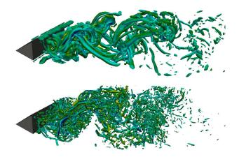
FIG. 3. Vortex shedding pattern for the cold flow. Top: Q-criterion for Case A at  $2.0 \times 10^6$ . Bottom: Q-criterion for Case B at  $2.0 \times 10^7$
