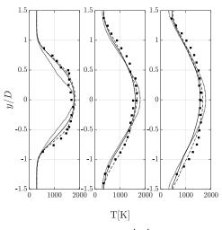
FIG. 6. Temperature profiles at  $(x_4, x'_4, x'_5 - \text{left to right})$ . Case A (solid line), Case B (dashed line), experimental data (black solid square) and reference data - two/step chemistry<sup>22</sup> (dotted line)
