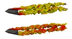
FIG. 5. Iso-surface of the progress variable at 0.5 for the reactive test case (colored by wrinkling factor). Top: Case A. Bottom: Case B
