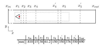
FIG. 1. A Mid-plane cut view of the domain in z-direction is presented, indicating all the positions where measurements are available. The axes origin is identified as the red dot. The dimension of the equilateral triangle is D = 0.04m, spanning throughout the width of the burner. The dotted lines indicate the location of the refined region for Case B.
