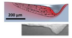
**FIG. 9.** Comparison of FE and experimental keyhole shapes. X-ray images were reprinted with permission from R. Cunningham, C. Zhao, N. Parab, C. Kantzos, J. Pauza, K. Fezzaa, T. Sun, and A. D. Rollett, Science **363**, 849–852 (2019). Copyright 2019, AAAS.
