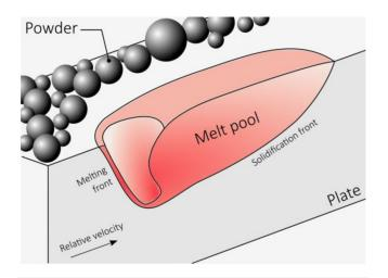
FIG. 1. Schematics of the melt pool in LPBF.
