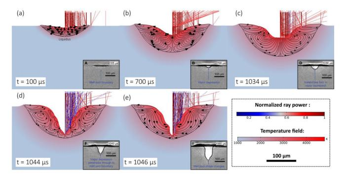
FIG. 3. Keyhole formation steps during stationary irradiation. (a) Conduction mode. (b) Forced conduction mode. (c) Vapor depression instabilities. (d) Keyhole mode. (e) Keyhole fluctuations. X-ray images were reprinted with permission from R. Cunningham, C. Zhao, N. Parab, C. Kantzos, J. Pauza, K. Fezzaa, T. Sun, and A. D. Rollett, Science 363, 849–852 (2019). Copyright 2019, AAAS.
