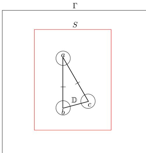
Fig. 3: The computational domain is delimited by an artificial boundary  $\Gamma$ . A side of  $\Gamma$  has a length of 60 nm. The cross sections are computed on a line  $S$  around the scatterer, which is approximately 20 nm away from it. The black-hole fluxes and energy are computed in small disks centered at each corner.
