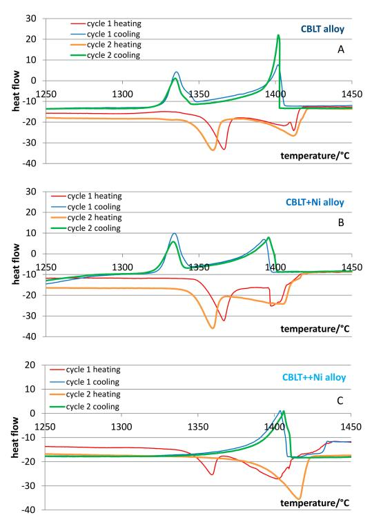
**Figure 2.** The differential scanning calorimetry (DSC) curves obtained for the two successive cycles (plotted as heat flow versus temperature): **(A)** the CBLT alloy; **(B)**: the CBLT+Ni alloy; **(C)** the CBLT++Ni alloy.
