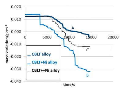
**Figure 7.** The cooling parts of the TG curves (plotted as mass variation versus time, after correction from the consequence of the air density variation): A: the CBLT alloy; B: the CBLT+Ni alloy; C: the CBLT++Ni alloy.
