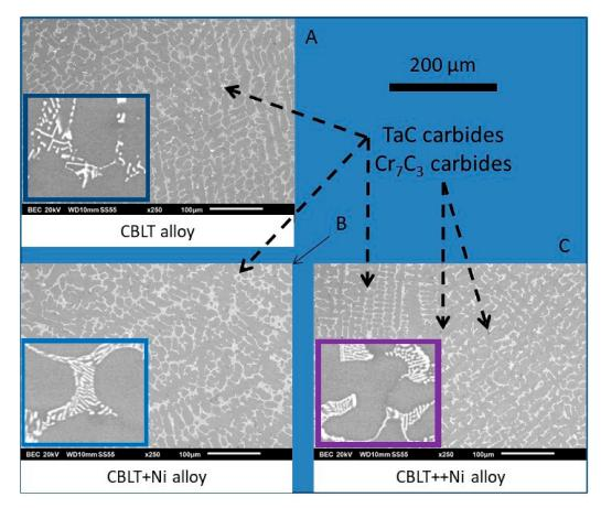
**Figure 1.** SEM/BSE microstructures of the three alloys in their as-cast states (large micrographs  $\times 250$ ; inserted micrographs  $\times 2000$ ): (**A**): the CBLT alloy; (**B**): the CBLT+Ni alloy; (**C**): the CBLT++Ni alloy.
