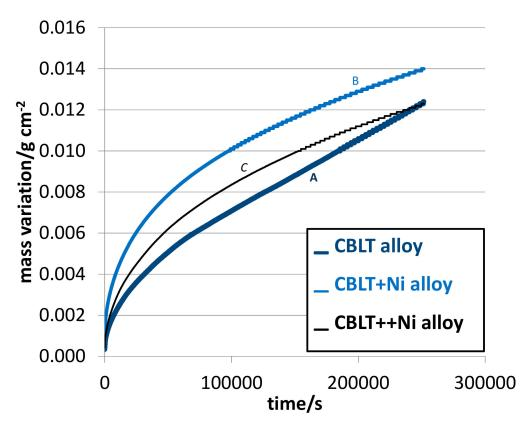
**Figure 6.** The isothermal parts of the TG curves (plotted as mass gain versus time): **A**: the CBLT alloy; **B**: the CBLT+Ni alloy; **C**: the CBLT++Ni alloy.
