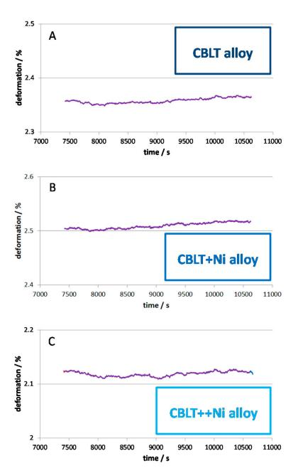
**Figure 4.** The isothermal parts of the TMA curves (plotted in the (deformation versus time) scheme): **(A)** the CBLT alloy; **(B)** the CBLT+Ni alloy; **(C)** the CBLT++Ni alloy.
