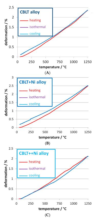
**Figure 3.** The thermo-mechanical analysis (TMA) curves obtained for three alloys (plotted in the (deformation versus temperature) scheme): (**A**) the CBLT alloy; (**B**) the CBLT+Ni alloy; (**C**) the CBLT++Ni alloy.
