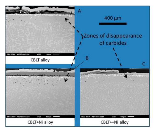
**Figure 8.** General view of the surfaces and subsurfaces affected by oxidation: **(A)**: the CBLT alloy; **(B)**: the CBLT+Ni alloy; **(C)**: the CBLT++Ni alloy.
