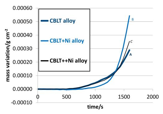
**Figure 5.** The heating parts of the thermogravimetry (TG) curves (plotted as mass gain versus time, after correction from the consequence of the air density variation); A: the CBLT alloy; B: the CBLT+Ni alloy; C: the CBLT++Ni alloy.
