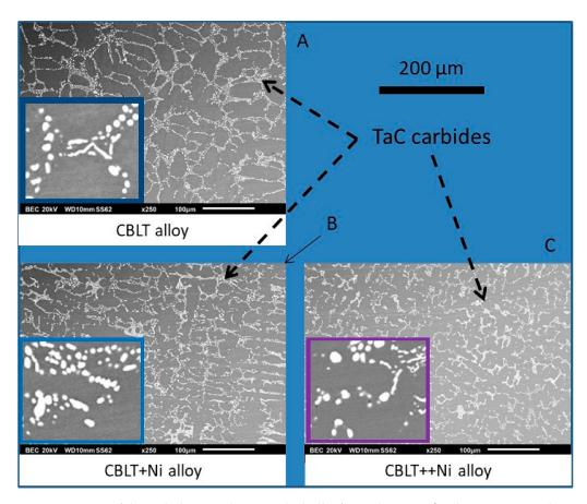
**Figure 10.** View of the carbides population in the bulk after 70 h at 1250  $^{\circ}$ C (large micrographs 250; inserted micrographs ×2000): (**A**): the CBLT alloy; (**B**): the CBLT+Ni alloy; (**C**): the CBLT++Ni alloy.
