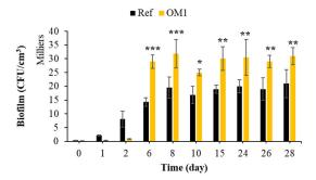
**Figure 16.** Quantification of bacterial biofilm on untreated mortars and mortars treated with formwork oil. Each experiment was performed in triplicate, and the error bars present the standard deviation of the values obtained. The experiments highlighted with asterisks differed significantly from the control (Bonferroni; \*: p < 0.05, \*\*: p < 0.01, \*\*\*: p < 0.001) at the indicated time.
