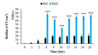
**Figure 12.** Quantification of bacterial biofilm on smooth and rough mortars. Each experiment was performed in triplicate, and the error bars present the standard deviation of the values obtained. Ref = control mortar; BM1 = biomimetic mortar prepared with CEM I. The experiments highlighted with asterisks differed significantly from the control (Bonferroni; \*\*\*: p < 0.001) at the indicated time.
