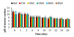
**Figure 10.** Evaluation of the pH of mortar surfaces. Each evaluation was performed in triplicate, and the error bars present the standard deviation from the values obtained. Ref = control mortar; CM = cured mortar; OM1 = oiled mortar prepared with CEM I; OM3 = oiled mortar prepared with CEM III; BM1 = biomimetic mortar prepared with CEM II; BM3 = biomimetic mortar prepared with CEM III.
