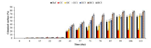
**Figure 17.** Quantification of marine fouler organisms using an image-analysis-based method. Ref = control concrete; CC = cured concrete; OC = oiled concrete; EC1 = ECOPODE™ concrete prepared with CEM I; EC3 = ECOPODE™ concrete prepared with CEM III; BC1 = biomimetic concrete prepared with CEM II, BC3 = biomimetic concrete prepared with CEM III. Each experiment was performed on 15 replicates, and the error bars present the standard deviation of the values obtained.
