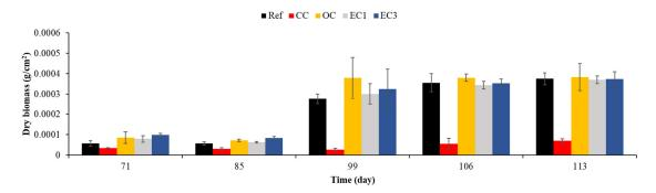
Figure 19. Quantification of marine fouler organisms using dry-weight biomass measurement. Ref = control concrete; CC = cured concrete; OC = oiled concrete; EC1 = ECOPODE<sup>TM</sup> concrete prepared with CEM I; EC3 = ECOPODE<sup>TM</sup> concrete prepared with CEM III. Each experiment was performed in triplicate, and the error bars present the standard deviation of the values obtained.
