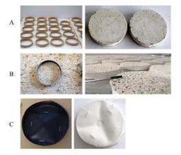
**Figure 4.** Preparation of concrete specimens. **(A)** Preparation of SS concrete specimens; **(B)** preparation of RS concrete specimens; **(C)** preparation of FPS concrete specimens.
