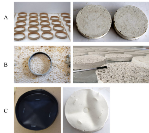
Figure 4. Preparation of concrete specimens. (A) Preparation of SS concrete specimens; (B) preparation of RS concrete specimens; (C) preparation of FPS concrete specimens.
