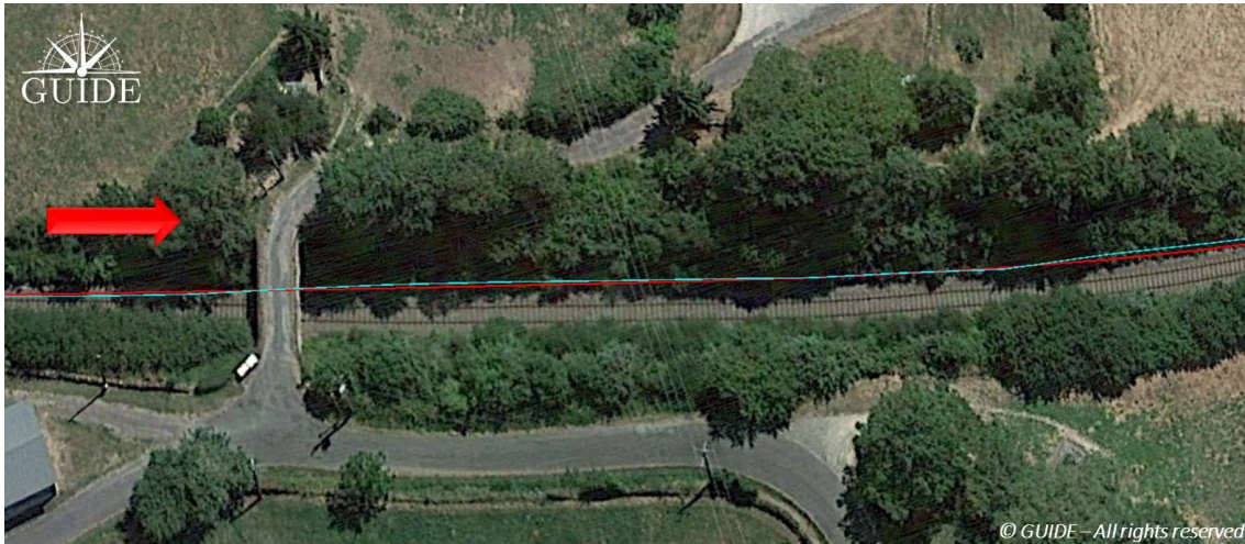
Figure 11: Single PVT track (cyan/blue) after a bridge crossing
