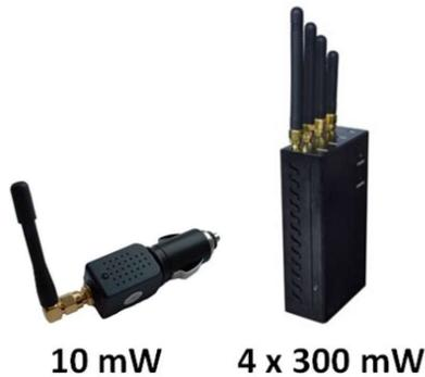
Figure 4.44 Typical in-car chirp jammers Personal Privacy Devices
