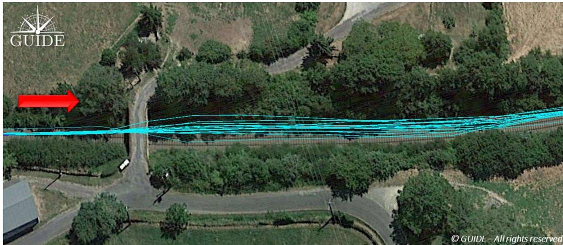
Figure 4.18 Multiple PVT tracks (cyan/blue) after bridge crossing
