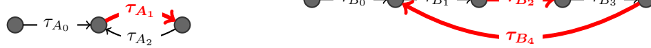
(a) Automaton A , allocated to core c_A , which describes a periodic behavior: after \tau_{A_0} has been taken, the sequence \tau_{A_1} and \tau_{A_2} is repeated.
