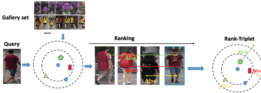
Fig. 1: Schematic illustration of Rank-Triplet. An image of a person of interest on the left (the query) is used to rank images from a gallery according to how closely they match that person. The correct match, highlighted in a blue box, can be difficult to find given the similar negative images, pose and viewpoint variations and occlusions. During training, we propose to estimate the importance of mis-ranked pairs by the gain of the evaluation measure incurred by swapping the rank positions and to weight the loss according to their importance. In this example, swapping the falsely ranked (positive) image on the right with the leftmost one would lead to the biggest improvement ( \Delta Eval ).
