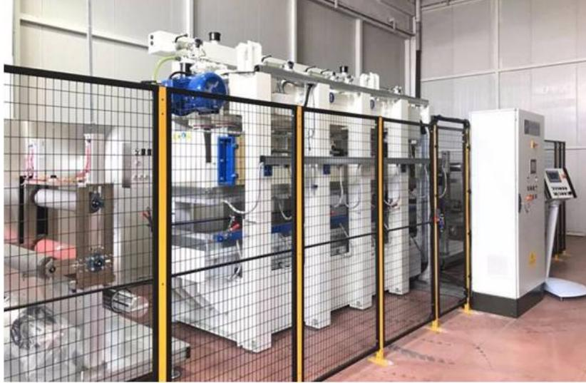
Fig. 14: The NOVOTECH press which produced the hybrid material
