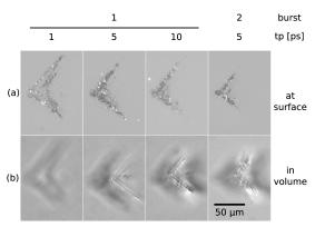
**Fig. 3.** Top views of permanent modifications (a) at the surface and (b) at a depth of 60  $\mu$ m within the volume of the glass with focal length f=10 mm, burst energy  $E_{\rm burst}=204$   $\mu$ J, and focus position  $\Delta z=200$   $\mu$ m for varying pulse durations  $t_p$  and burst configurations. Both (a) reflected and (b) transmitted light microscopy were used for optimal contrast; still the blurred image of the surface modification can be seen in (b).
