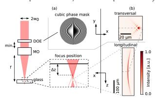
**Fig. 1.** Experimental 2f-setup (a) used for creating an Airy–Gauss beam (see text for details) and intensity profiles (b) according to Eq. (1) for f = 10 mm. Throughout the paper, the focus position is given as the shift  $\Delta z$  of the glass surface with respect to the focus position in air (red dotted line).
