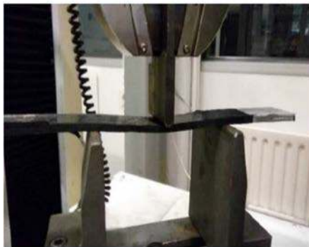
(a) Three-points bending bench
