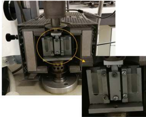
(b) Metravib DMA Bench
