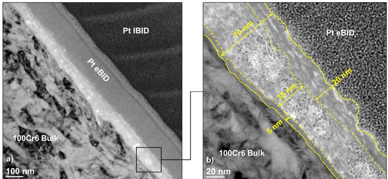
**Figure 7:** High magnification (x60,000) TEM observations in the bright field of the lamella T1b-L. A modified layer is fixed on the 100Cr6 bulk with a homogeneous depth ranging between 50 and 70 nm along the lamella. At the highest magnification, from the bulk to the Pt eBID layer, we can observe a thin interface layer; a larger amorphous phase containing nanoparticles; and a last amorphous layer.
