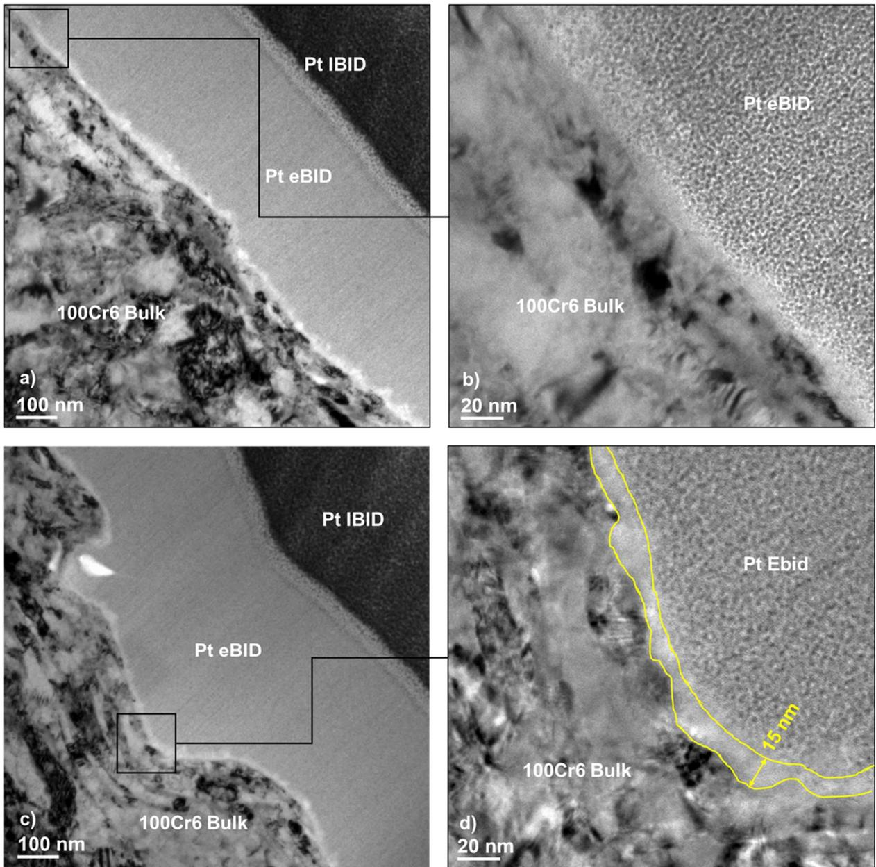
**Figure 8:** High magnification (x60,000) TEM observations in the bright field of the lamella T1C-L at two points along the FIB lamellae. A thin modified layer is fixed along the 100Cr6 bulk with a homogeneous depth about 6 nm along the lamella. At the highest magnification, the layer appears to not be developed in the b) section, whereas it is definable on the d) section.
