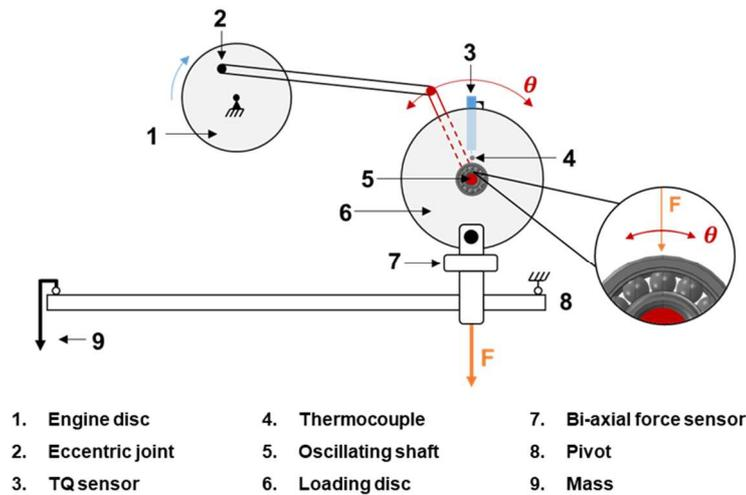
Figure 1: Scheme of the "R2" test bench
