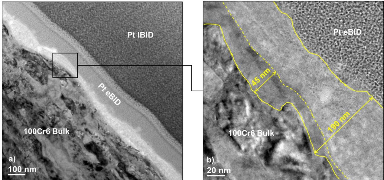
**Figure 9:** High magnification (x60,000) TEM observations in the bright field of the lamella T2b-L. A modified layer is fixed along the 100Cr6 bulk with a homogeneous depth about 100 to 205 nm along the lamella. At the highest magnification, from the bulk to the Pt eBID layer, an interface layer is observable, followed by a larger amorphous phase containing nanoparticles.
