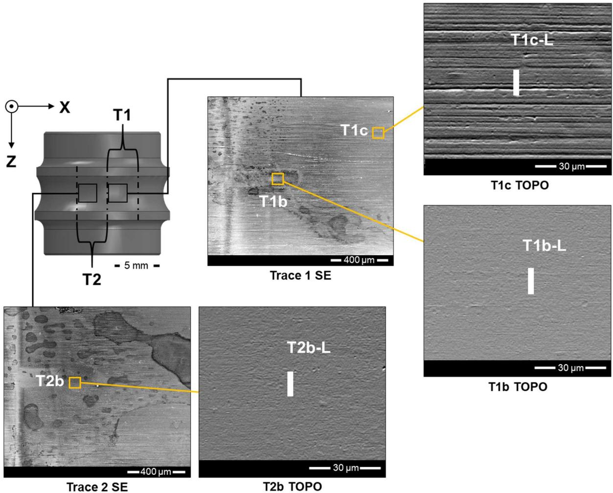
**Figure 4:** SEM (tension 15 keV, spot 5, WD 10.8 mm) observations of the rolling traces T1 and T2. The magnifications show details of the smoothed superficial layer at the reversing areas T1b and T2b; another magnification shows a detail of the plasticized area T1c at the central zone of the contact trace.
