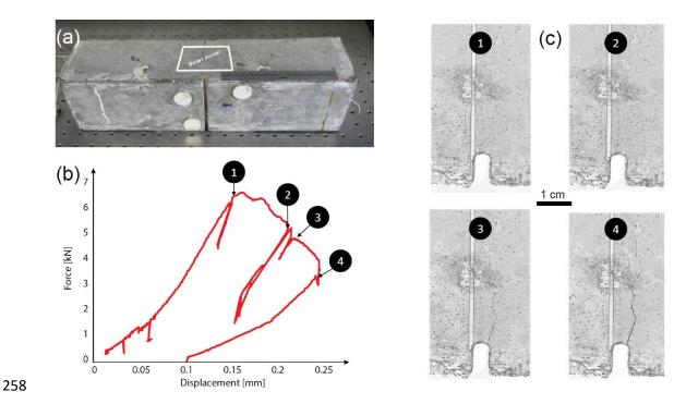
Figure 1. (a) Image of the sample showing where the acoustic scan zone is located. (b) Force/displacement curved recorded during the mechanical test. 1 to 4 symbols represent the times when the notched region was photographed. Corresponding images are shown in (c).
