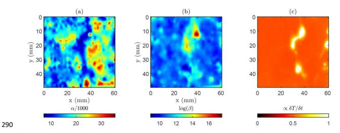
Figure 4: Experimental images of the cracked region. (a) Nonlinear  $\alpha$  parameter. (b) Harmonic generation ( $\beta$  parameter). (c) Vibro-thermography image: first derivative of the temperature with respect to time (the reader can refer to [23] for more details).
