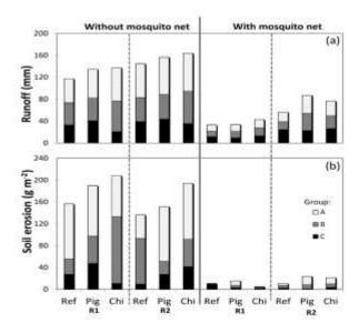
**Fig. 3** Bar plots showing cumulated **(a)** runoff depth and **(b)** soil erosion from the eighteen  $0.5\text{m}^2$  sub-plots (i.e. nine without plus nine with mosquito net) divided into triplicated treatment groups (A, B, C). Controls with no amendments (Ref) or amended with pig manure (Pig) or poultry manure (Chi). Measurements were conducted during the first rainfall simulation (R1, before manure application) and the second rainfall simulation (R2, after manure application)
