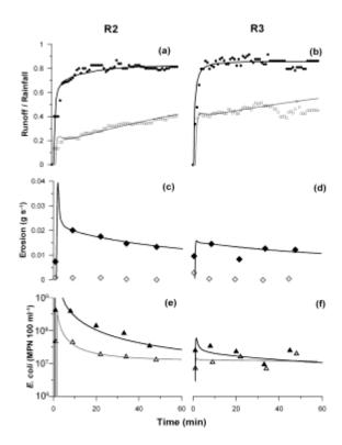
**Fig. 5** Evolution over time on plot Chi A of the runoff coefficient (Runoff/Rainfall) obtained during R2 (a) and R3 (b); the sediment outputs obtained during R2 (c) and R3 (d); *E. coli* concentrations obtained during R2 (e) and R3 (f). In each figure, empty and filled symbols correspond to the experimental results for the sub-plots with and without a mosquito net, respectively. Solid lines correspond to the modelled evolutions with mosquito net (grey) and without mosquito net (black)
