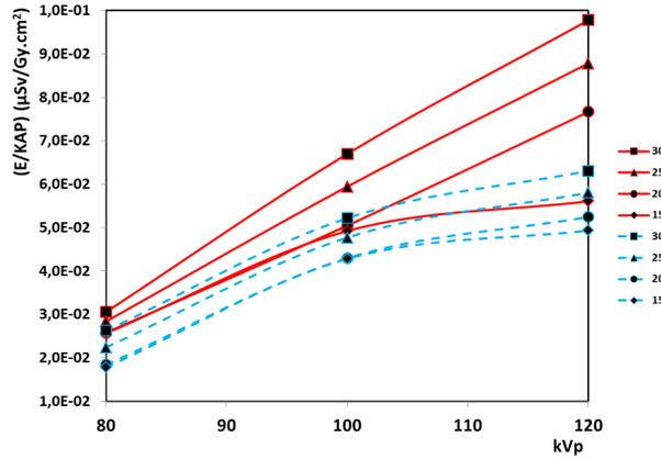
Figure 4. Occupational effective dose function of kVp for different FOV:  $15 \times 15 cm^2$  /  $20 \times 20 cm^2$  /  $25 \times 25 cm^2$  /  $30 \times 30 cm^2$  (continuous: main operator, discontinuous: assistant operator).
