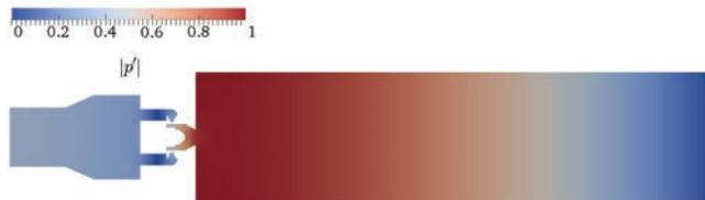
Figure 15: Acoustic mode obtained with Helmholtz solver.
