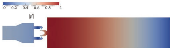
Figure 15: Acoustic mode obtained with Helmholtz solver.
