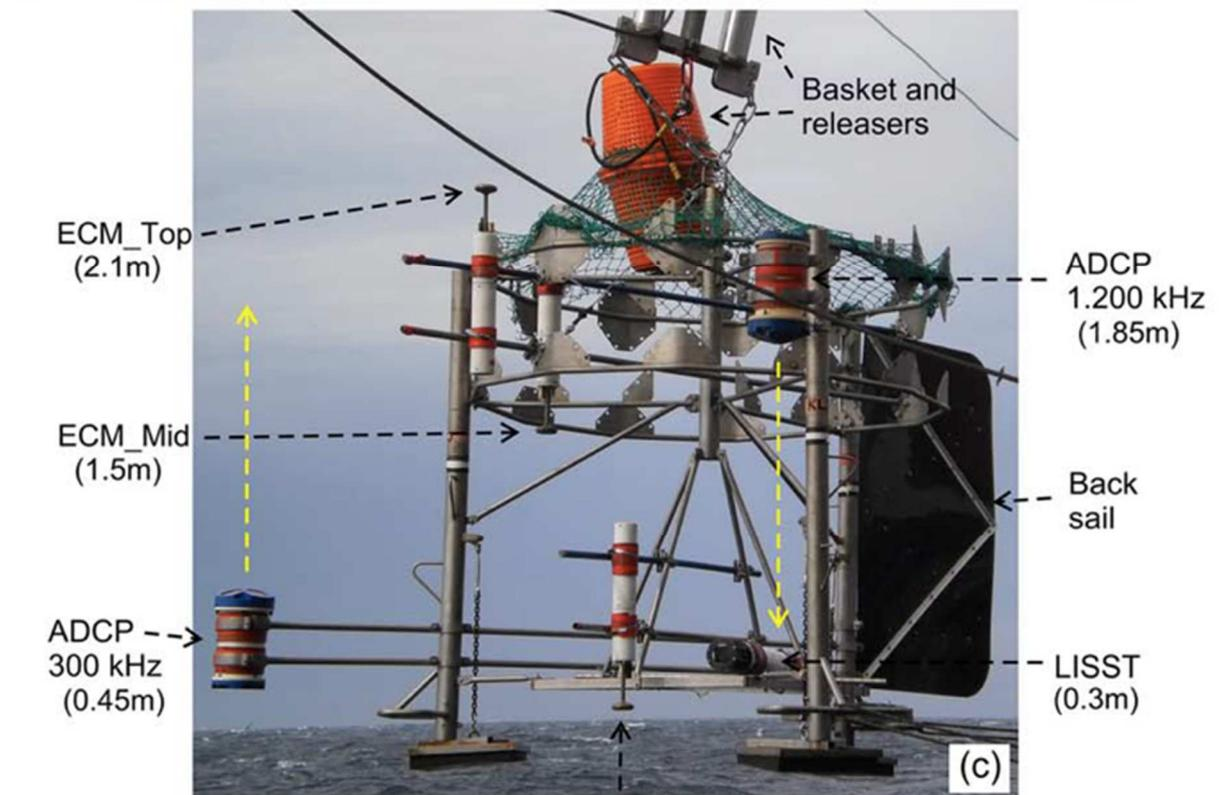
Figure 3. Photograph of a seabed lander and its instrumentation. Distance of each instrument from the bottom of the lander is also indicated. From Zhang et al. (2015), with permission from John Wiley and Sons.
