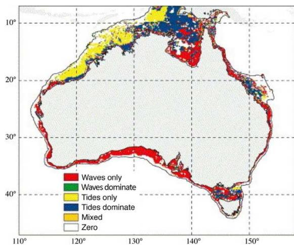
Figure 8. Regionalization of the Australian continental shelf based on estimated exceedance of the velocity thresholds for sediment mobilization caused by waves and tides. Adapted from Porter-Smith et al. (2004), with permission from Elsevier.
