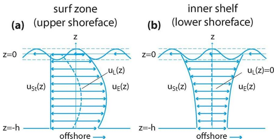
Figure 6. Two-dimensional ( $x, z$ ) wave-driven circulation typically observed (a) inside the surf zone (US) where the onshore Lagrangian Stokes drift  $u_{St}(z)$  is uniform in depth and the offshore wave-driven Eulerian undertow  $u_E(z)$  is parabolic, resulting in a vertical imbalance in the net mean flow,  $u_L(z) \neq 0$  (dashed line); (b) over the inner shelf (LS), where the onshore Lagrangian Stokes drift  $u_{St}(z)$  and the offshore wave-driven Eulerian undertow  $u_E(z)$  cancel,
