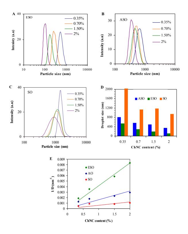
**Figure 2.** (A,B,C) Droplet size distribution for ESO, ASO and SO, emulsion at different ChNC content (wt%). (D) Mean droplet size of ASO, ESO and SO emulsion as a function of amount of added ChNCs, and (E) evolution of 1/D *vs* ChNC content for the corresponding emulsion. Oil concentration: 15 wt%.
