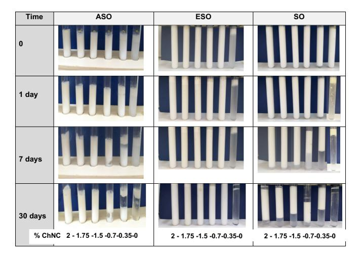
**Figure 7.**Change in the aspect of the emulsion with storage time, according to the oil type and ChNC content (from left to right): 2, 1.75, 1.5, 0.7, 0.35 and 0 wt% ChNCs based on the water phase). Oil fraction: 0.15.
