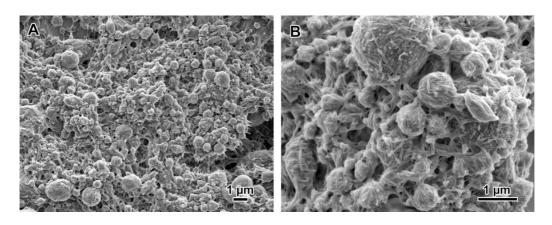
**Figure 6.**A,B) SEM images of an ASO emulsion stabilized with 1.5 wt% ChNCs. The emulsion containing 1% Irgacure 184 photoiniator was exposed to UV-light for 1 min to induce crosslinking in oil droplets.
