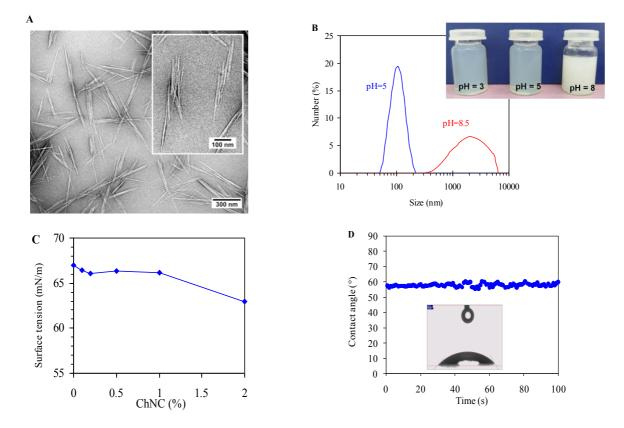
**Figure 1.** (A) TEM image of a negatively stained preparation of ChNCs at pH 6; (B) particle size distribution at pH 5 and pH 8.5; (C) surface tension *vs* ChNC content, and (D) contact angle of water *vs* time on a ChNC film.
