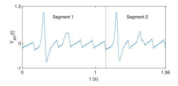
Fig. 2: Generated synthetic signal modeling an ECG with AF patterns plotted in time domain, where  $t=m/F_s$  are the time values in seconds and  $Y_{AF}(t)$  is the amplitude.
